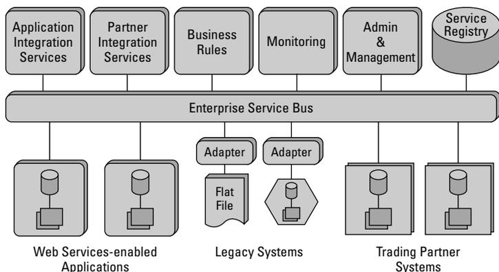
**Figure 5-2:** The Enterprise Service Bus architecture
