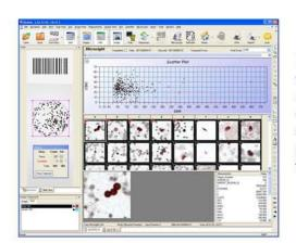
High resolution images are evaluated in the Review gallery. The system precisely relocates to any object with a single click for viewing through the microscope oculars. The gallery, slide map and plotting tools are all interactively linked for easy sorting and full analysis.
