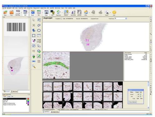
Ariol gives you speed and accuracy that cannot be achieved with manual analysis. The system quickly and accurately quantifies the number of positively stained vessels and their density per area is expressed in square microns. The area of staining, and of the lumen if present, is calculated for each vessel.
